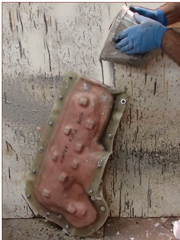
FIGURE 7-60: Pouring a casting
