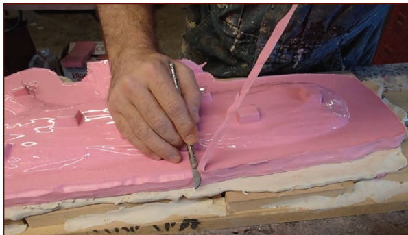
FIGURE 7-35: Cleaning up the edge of the rubber
