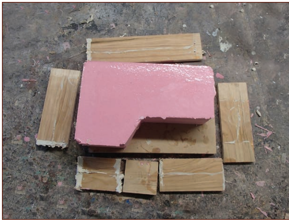
FIGURE 7-12: The disassembled mold box
