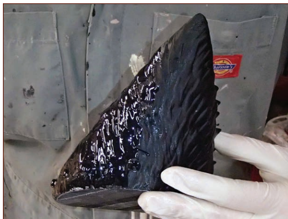
FIGURE 4-7: Using a specialized self-leveling resin to fill the build lines for the 3D printed ears
