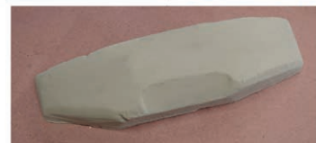
FIGURE 9-4: Pulling a plaster copy of the forming buck from a formed sheet
