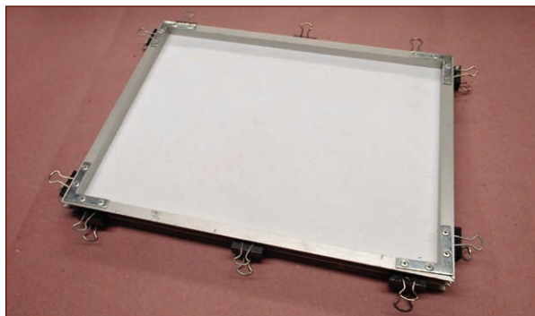
FIGURE 10-36: The plastic sheet in the clamping frame
