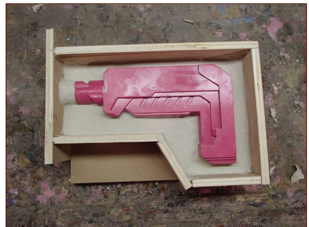
FIGURE 7-5: Filling in the area around the prototype with more clay
