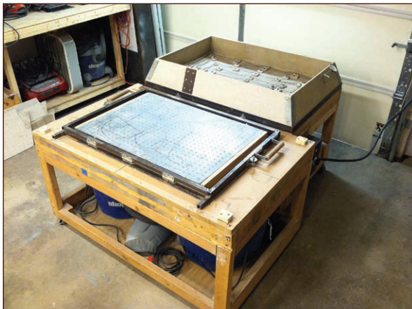
FIGURE 10-13: A typical, homemade side-by-side vacforming machine made by Sean Bradley of Sean Bradley Studios
