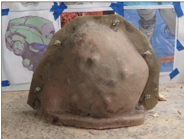
FIGURE 8-36: The reassembled mold; ready to roll
