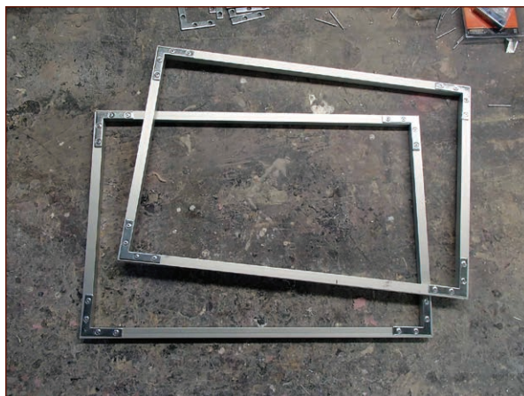
FIGURE 10-7: Boom! Clamping frame
