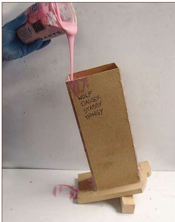
FIGURE 6-27: Pouring rubber with the mold box tipped slightly to allow bubbles to rise up and away from the prototype
