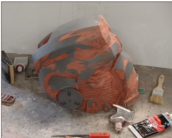
FIGURE 2-54: A few tiny holes filled with spot putty
