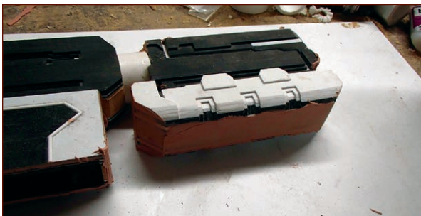
FIGURE 1-71: The nearly finished shape of the forward body attached to the front of the main body
