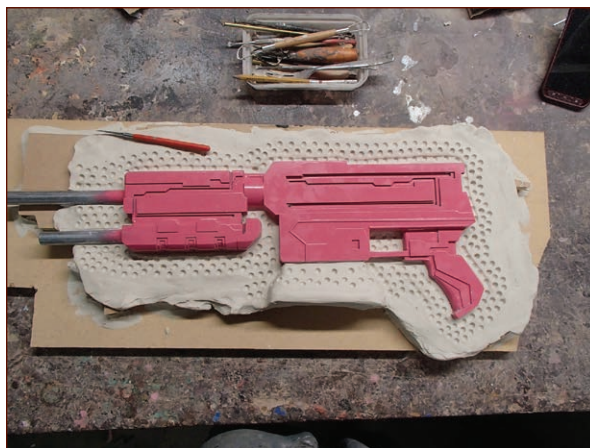
FIGURE 7-25: The dimpled clay bed
