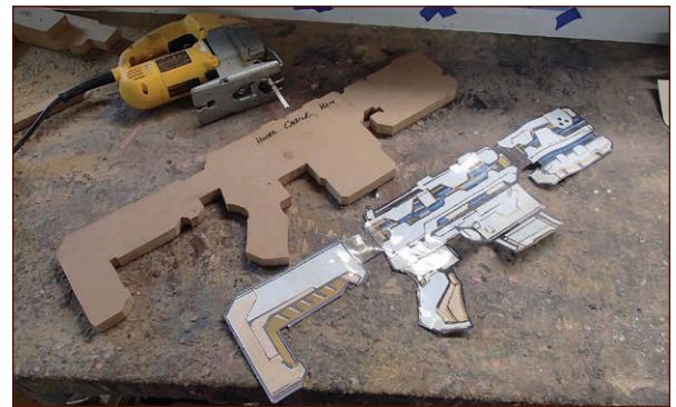
FIGURE 1-52: The jigsaw is the easy way.
