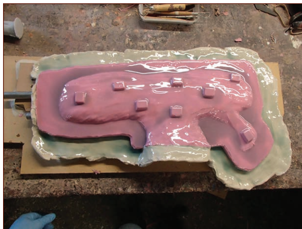
FIGURE 7-36: A coat of fiberglass resin painted onto the silicone and the clay bed
