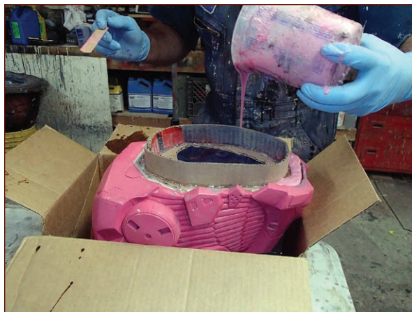
FIGURE 8-5: Filling the undercuts with silicone while the prototype is upside-down
