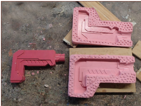
FIGURE 7-13: The demolded prototype
