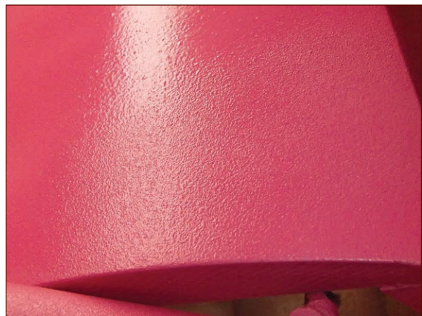
FIGURE 11-12: This surface might be okay for citrus fruits, but not for a glossy coat of paint
